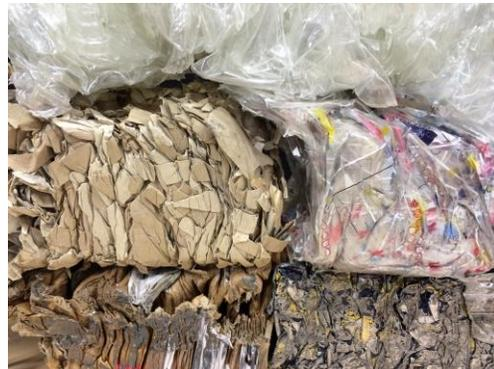
*Brickman briquettes: volume reduction up to 20:1*
