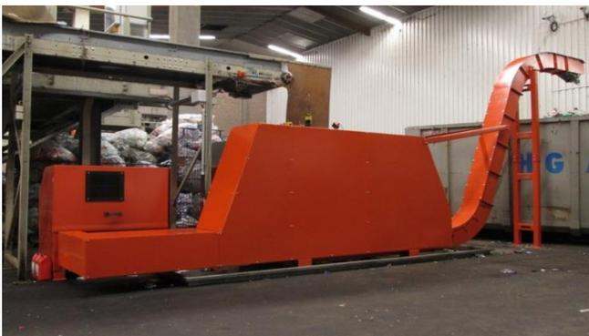
*Brickman 2000K has the capacity to process up to 25 000 empty PET bottles per hour*
